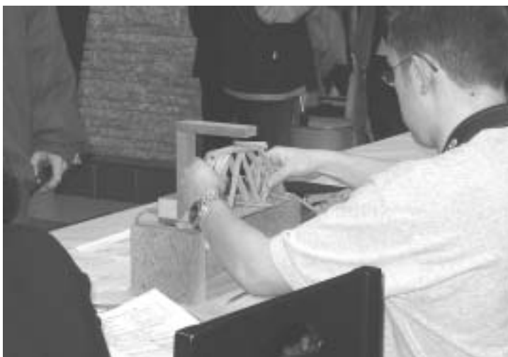
Spaghetti Bridge specifications are checked before load testing
